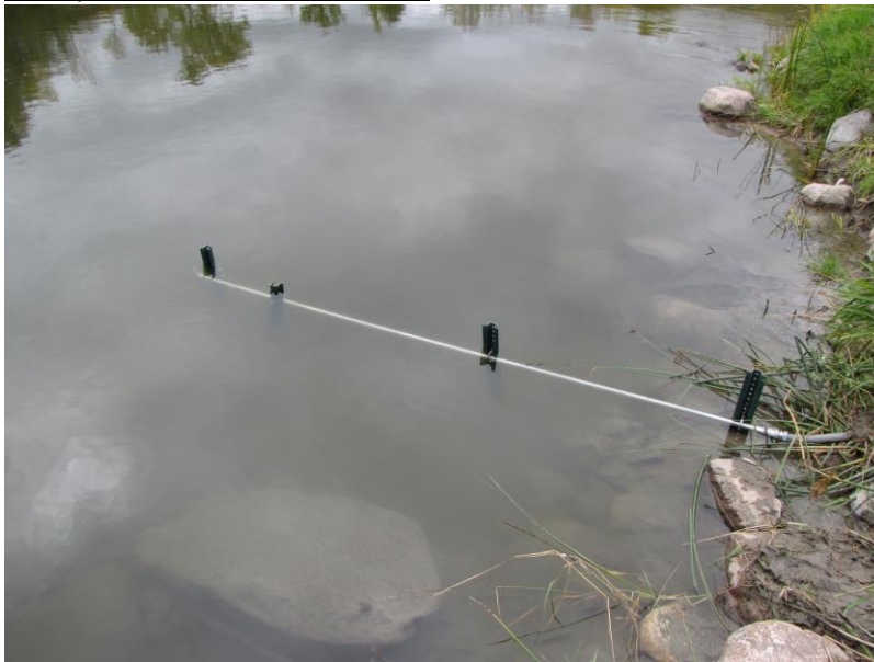
Example of bubbler line in water
