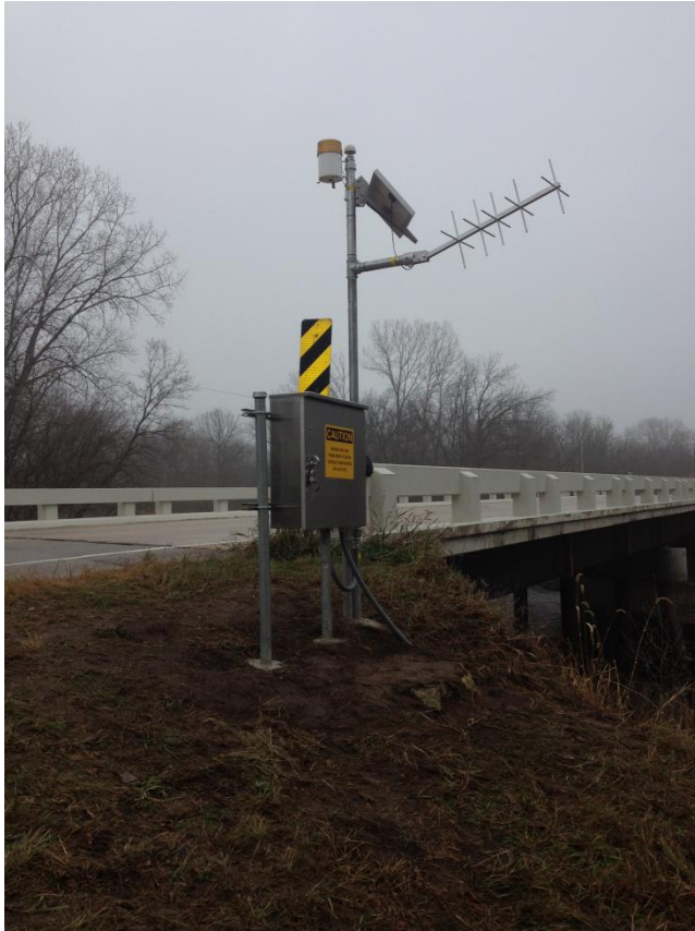
Example monitoring station cabinet
